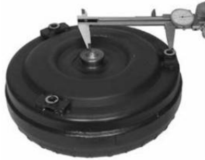
Bolt Radius (x 2 = Bolt Circle) Center of Pad to Center of Pilot
