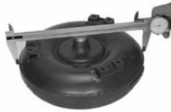
Diameter - Overall Outside of Conv. (Not Ring Gear)
