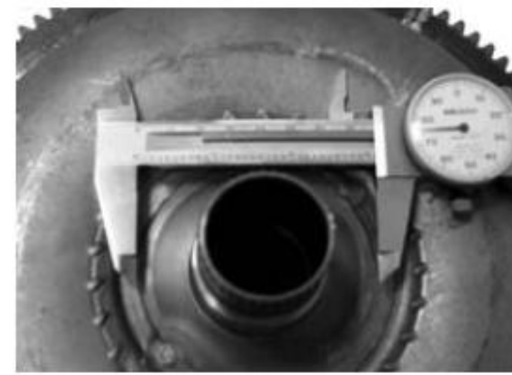
Hub Flange Outside of Flanged Area
