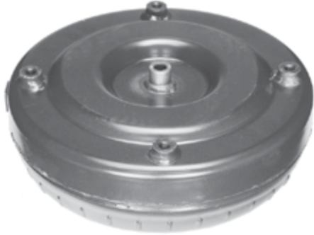
Early front cover with 'hollow' style pilot
