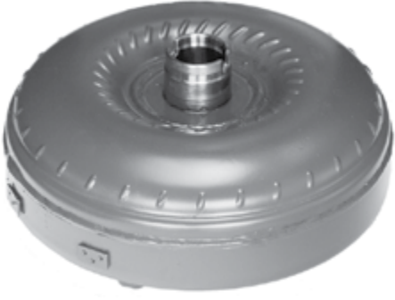
Late impeller with 2 rows of ribs
