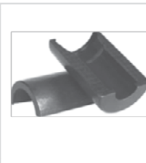
T-3211 Removes Output Shaft Bearing Cone From Rear Carrier Fits 93-Up 42LE Use with Bearing Remover T-1432
